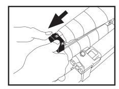
3. Remove the end cap located by the end of the valance. You will see two more screws, remove along with the plug/bung.
