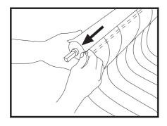
9. One more screw to remove, located by the end of the fabric/roller. This keeps the fabric in place.
