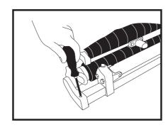
19. Finally, install the side awning bar back on, tighten up two screws front and back of the bar.
