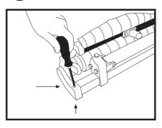
2. Remove two screws located at the front and back of awning bar. NOTE: usually hidden under a sticker.
