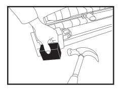
5. Use a wooden block and hammer the side awning bar. This will loosen the end bar, you should be able to pull the bar off with ease.
