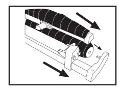
15. Slide the roller/fabric back into the frame. NOTE: Check to make sure the awning arms are still tied up so it wont get in the way.
