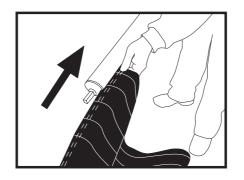
11. Replacing awning fabric cover. Slide the fabric back into the roller along the groove.
